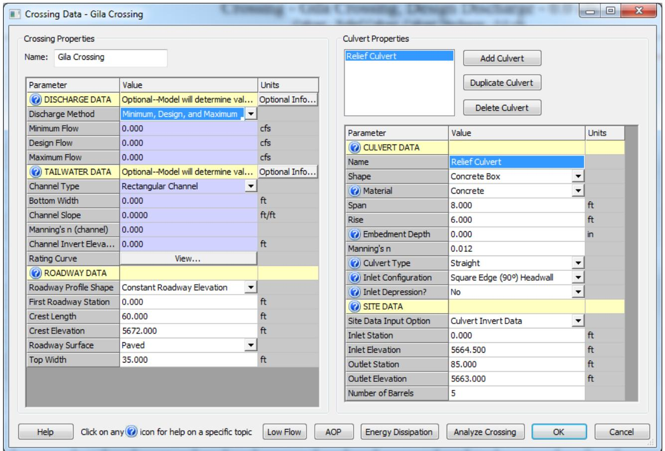
Figure 5 HY-8 Crossing and Culvert Inputs
