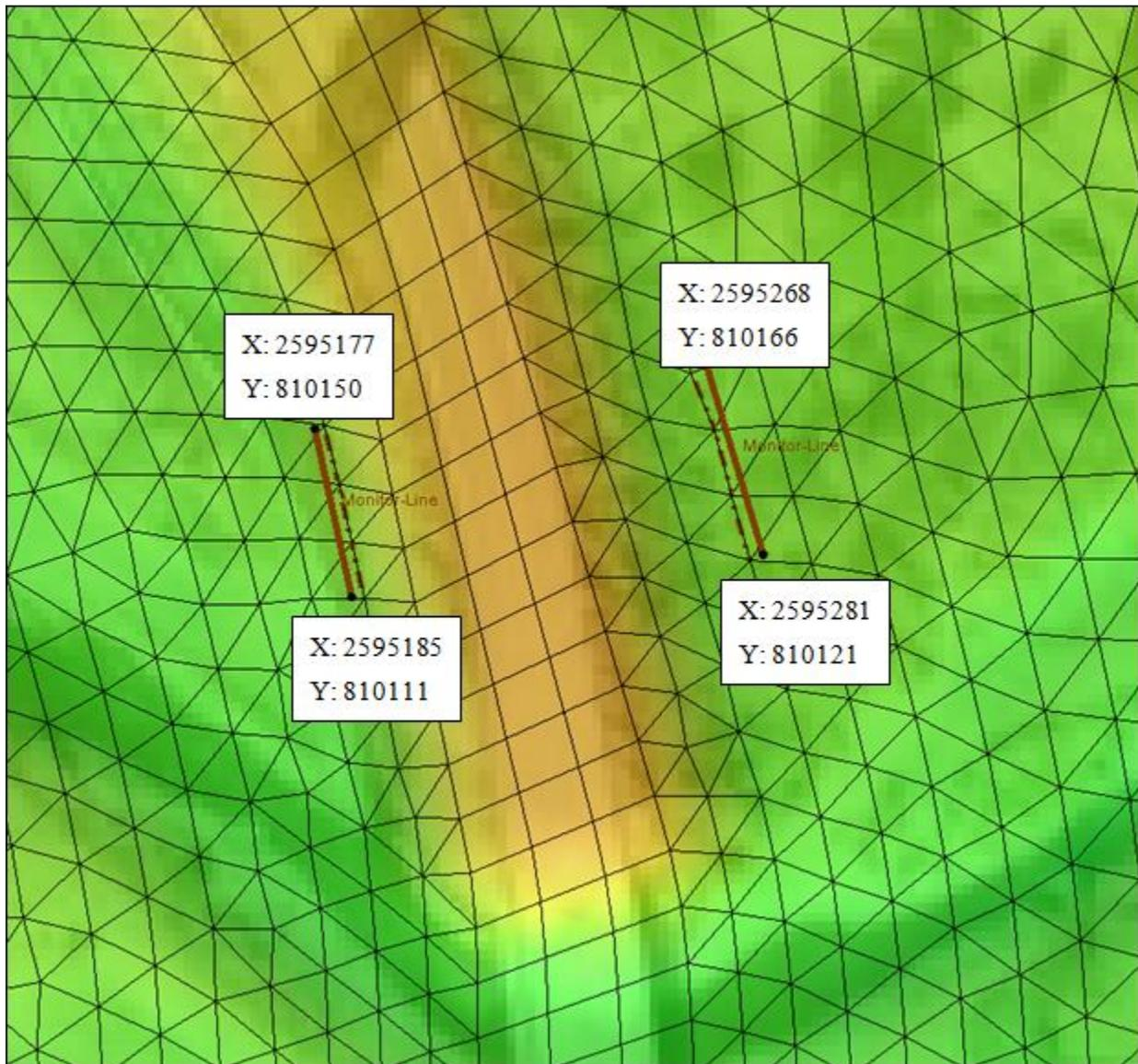
Figure 4 Coordinate Location of Arc End Nodes
